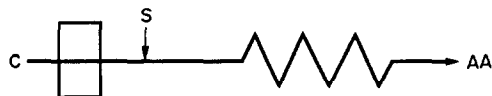
Fig. 1. Single line manifold. C is a distilled water carrier stream, S is the sample injection valve and AA is the model 5000 spectrometer. The connection between the valve and the detector was the minimum length of tubing possible.
